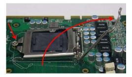
3. Lift the load plate to uncover the socket.
