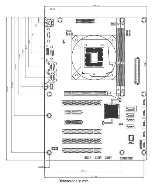
Figure 1-2: IMB-M40H Board Dimensions
