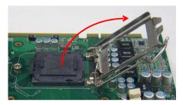
4. Remove the plastic protective cover from the socket. Note the locations of the alignment keys (A) and Pin 1 indicator (B).
