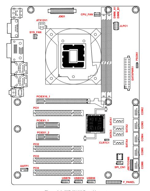
Figure 2-2: IMB-M40H Board Layout
