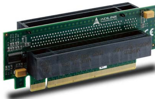
PCIEx16-to-two-x8 Adapter Card (Model: P16TO28, Part No.: 91-79301-0010)
